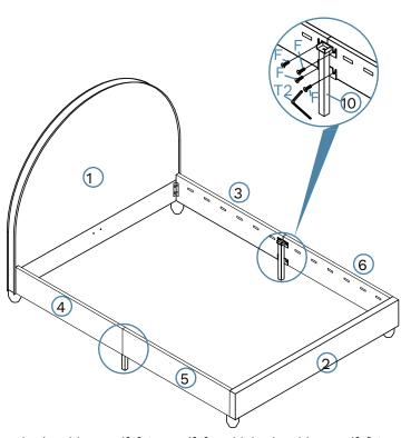
Join the side panel[3] & panel[6] and join the side panel[4] & panel[5] together with 2x legs(10) and secure with 8x 20mm bolts (F), Tighten with Allen Key (T2).
