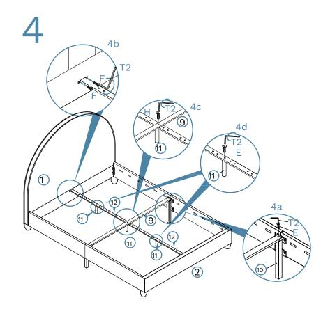
**4a:** Insert panel [9] and sit on top of the connector (10) and secure with 2x 25mm bolts (E). Tighten with Allen Key (T2).
