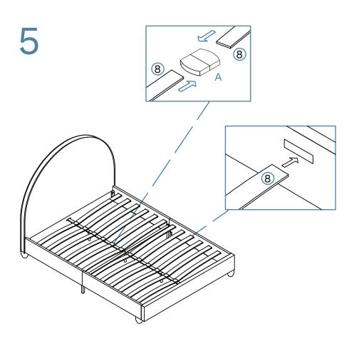
Join the bed planks together in the middle of the frame using 12x double caps (A). Insert the end of the planks into the bed frame as shown and attach the double caps (A) into panel [8]. Make sure the double caps (A) click securely into place.
