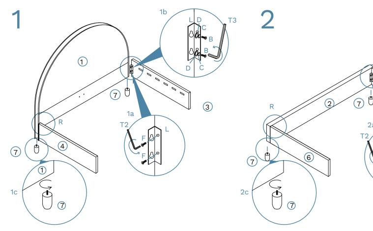
**1a:** Attach 1x left plate(L) to panel[3] and 1x right plate(R) to panel[4] and secure with 4x 20mm bolts(F). Tighten with Allen Key (T2).
